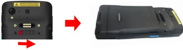
2. Grab the battery cover from the groove and remove it upwards.
